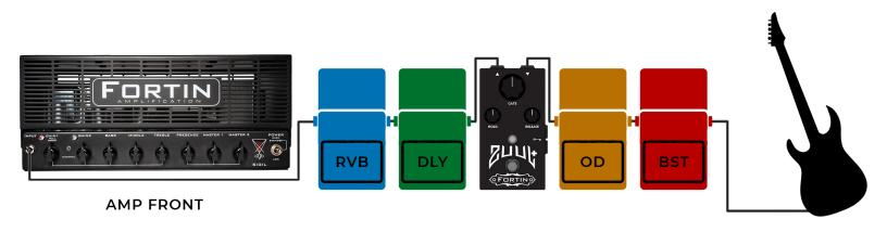
**WARNING:** 2 Cable Method will result in the Zuul responding to signal affected by pedals or signals before the Zuul.
